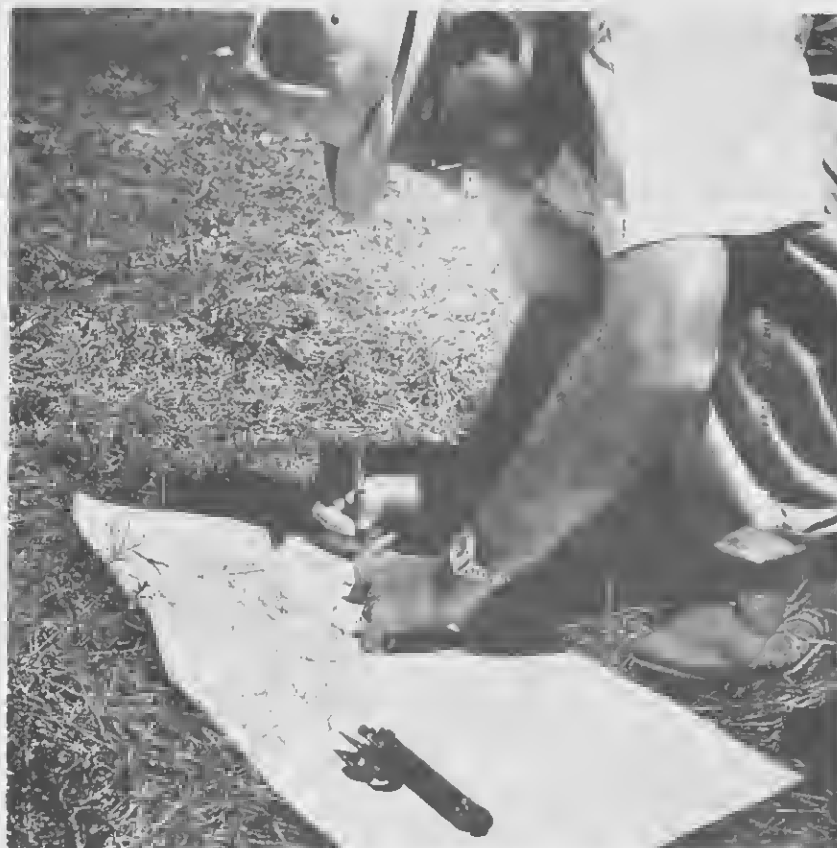
A TERRACE HEIGHT is carefully marked on a topographical map. Later Dr. Alexander will draw another map and incorporate his measurements.
